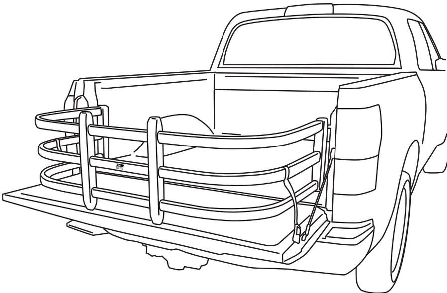
**BEDXTENDER HD<sup>TM</sup> shown assembled and installed on truck.**
