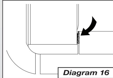
the inside surface of the tailgate. Make sure the Track End Cap Metal Blocks contact the Tailgate Extrusion End Caps (**Diagram 16**). Note that if the Tracks are not positioned as shown, the Latch Mechanism will not function correctly.
