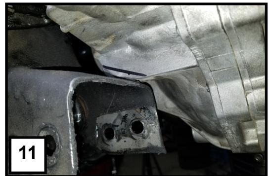
24. Attach the skid plate using OEM hardware. Do not install the main front bolt. The skid plate will be between the gravel guard and frame.
