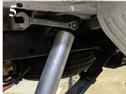
c) Remove the bolt attaching the front of the leaf spring and allow the spring to droop. This relieves the tension on the frame. **(PHOTO 6)**
