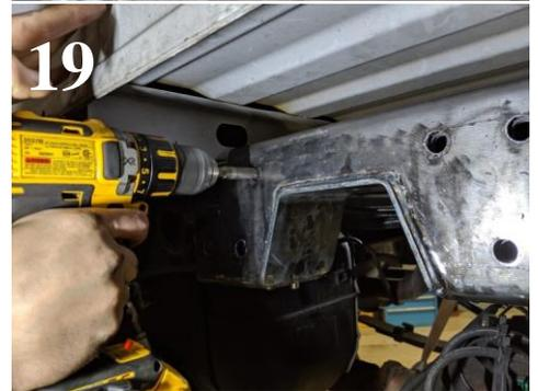
e) Once the holes are drilled, loosen the top and bottom bolts currently holding the backing plate into the shell, until the backing plate is allowed to move. Insert the Bolts through the Front of the shell.
