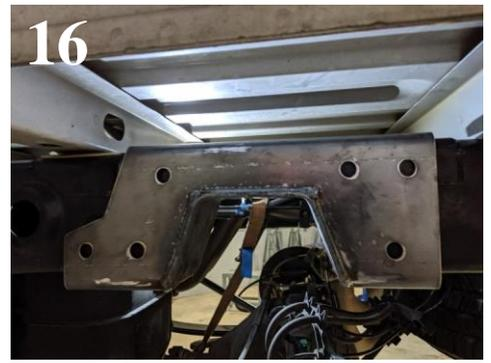
b) Insert the backing plate and attach the bolts. Tighten them to about 20 ft-lbs. or enough to hold the backing plate in firmly. The backing plate is there as a guide for the holes to line up concentrically. **(PHOTO 17)**
