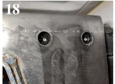
d) Drill pilot holes first with a smaller drill bit (this will also ensure the holes will be concentric from front to back), then either increment drill bits to enlarge the hole or use a step bit. Do not rush this process as overheating the metal will cause poor finish on the holes and dull drill bits. **(PHOTO 19)**
