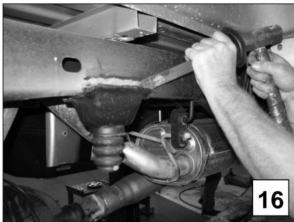
7c) Use an abrasive grinder to remove the excess material on the frame once the bracket has been removed. Use black spray paint to protect the raw exposed metal.
