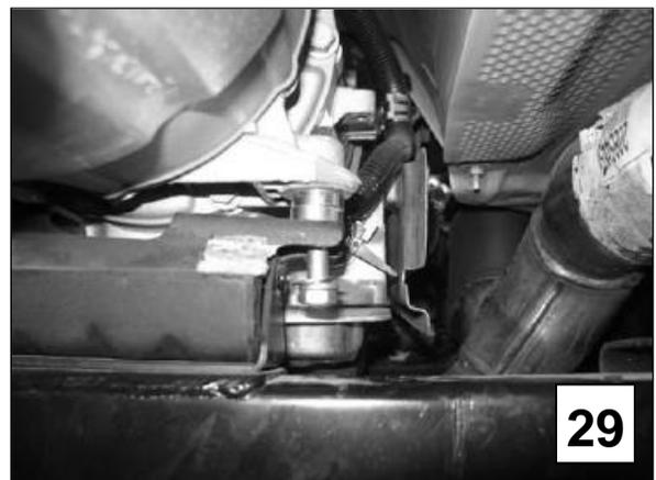
11d) Insert the BELLTECH Transmission spacers supplied, 2 per side. Re-attach the isolator to the transmission with the supplied hardware. (**Photo 29**)
