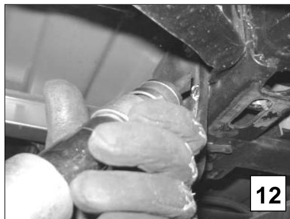
**NOTE:** If the rivets heads are not easily chiseled off, the cut thru the center is probably not deep enough. Increasing the depth of the slot thru the center will decrease the time it takes to remove the rivets. DO NOT cut all the way through the hanger bracket.
