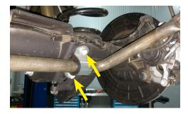
14. Remove the nuts and bolts from the rear of the upper and lower control arms to disengage from the axle side. Do not remove the frame side.
