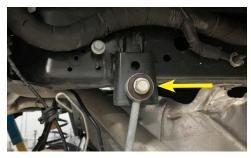
13. Remove the sway bar pivot bushing bracket bolts and remove the sway bar assembly from the vehicle.
