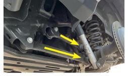
15. Lower the axle and remove both rear springs and rubber isolators from the vehicle. Mark the isolators to show how the locating tabs where seated spring pocket and where the original spring was positioned in the isolator.
