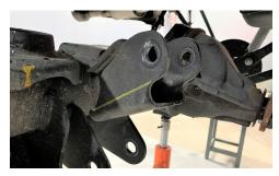
17. Cut off the lower end of the upper control arm brackets with a cutting tool. Do not cut into the axle. Paint over exposed metal to prevent rust/corrosion.
