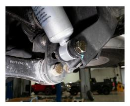
37. Torque all M16 x 2.0 nuts and bolts used to retain the control arm drop brackets to 111 ft lbs. + 110 $^{\circ}$  turn.
