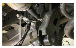
12. Disconnect the sway bar end links upper bolts from the frame.
