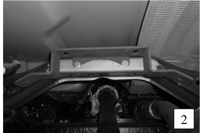
3b) Bolt Belltech CCB bracket on to crossmember (Photo 2) Note: This position is reverse mounted from final position to allow for marking crossmember for cutting.
