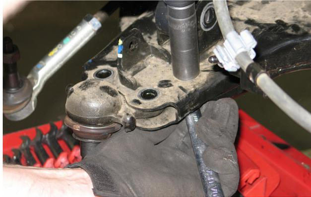
20. To install the new Belltech lower ball joint, the lower sway bar end link bracket must be removed. Using a reciprocating saw or a cutting wheel, remove the bracket, cutting it flush to the top of the lower control arm.
