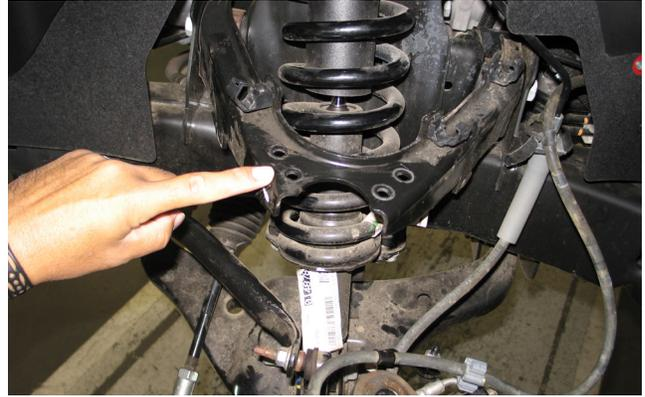
18. Remove the 21mm bottom strut bolt to disengage it from the lower control arm
