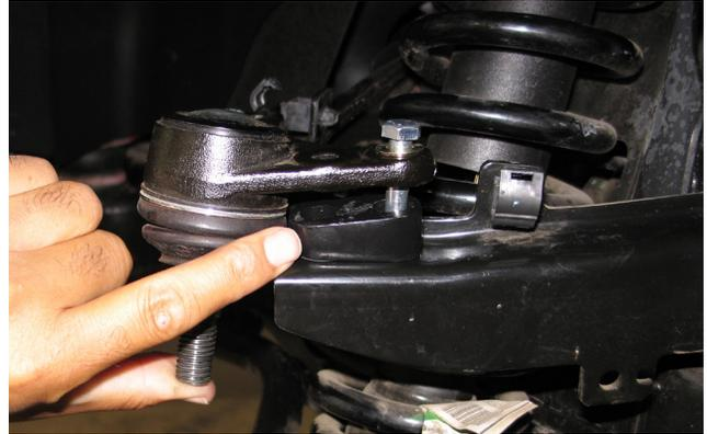
23. The bottom spacer is placed on the underside of the upper control arm.
