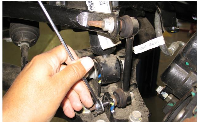
11. Break loose but do not completely remove the 21mm tie-rod ball joint nut. Ensure there are few threads engaged to help unseat the tie-rod ball joint.
