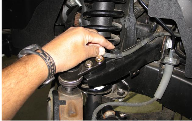
35. Place a jack under the lower control arm to raise the suspension to simulate (load) the vehicle weight on the ground.
