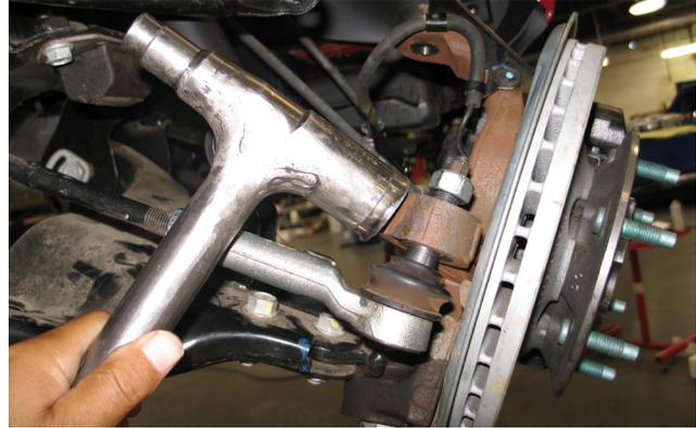
13. Place a floor jack under the lower control arm and lift until a slight compression of the suspension is achieved.
