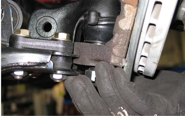
30. Attach the lower strut mount to the lower control arm with the original bolt and nut. Do not torque yet.
