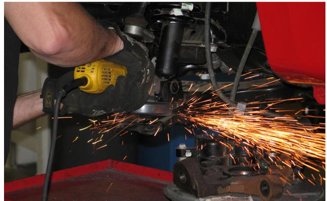
21. Use a grinder to smooth the cut surface. Wipe the area down with a cleaning solvent and spray paint the exposed metal.
