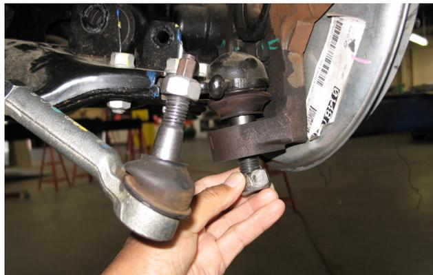
16. Remove upper and lower ball joint nuts to detach the spindle from the control arms.
