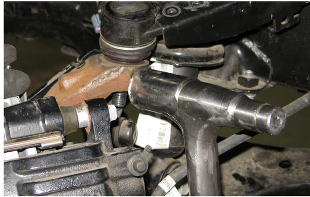
15. Break loose but do not completely remove the 27mm lower ball joint nut. Ensure there are few threads engaged to help unseat the ball joint. With a large hammer, strike the side of the spindle boss until the lower ball joint is dislodged.
