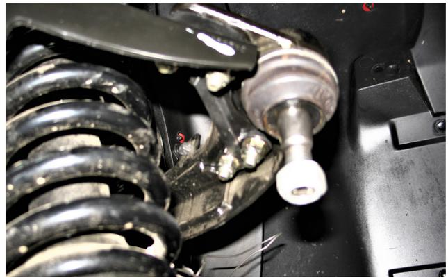
24. Fasten the upper ball joint assembly with four 5/16"-24 X 2.0" hex head bolts, four flat washers, and the four 5/16"-24 lock nuts. Torque to 12 ft lbs.
