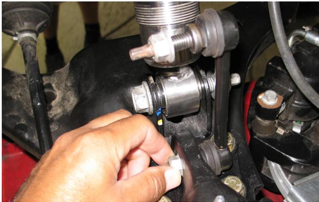
32. Attach the upper end link to the sway bar with the original nut. Do not torque yet.
