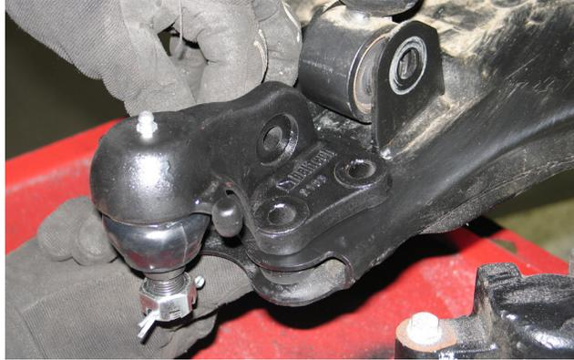
27. Fasten the lower ball joint assembly with four 7/16"-20 X 2.25" hex head bolts, four flat washers, and the four 7/16"-20 lock nuts supplied with the lower ball joint. Torque to 44 ft lbs.
