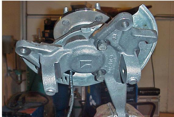
32. In sequence, tighten the locknut and the hub bolts until the hub flange is flush against the brake backing plate and the hub face of the spindle. Torque locknut to 34 ft lbs. Verify that adequate clearance exists between the backside of the hub flange and the threaded stud. Torque the original hub bolts to 70 ft lbs.
