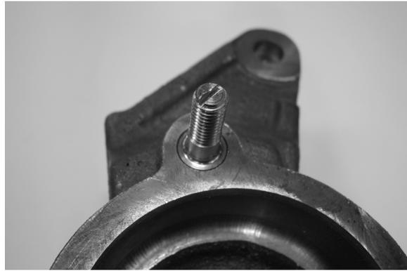
27. Place the brake backing plate onto the hub face of the lowering spindle in the same orientation as removed. Be sure to have the inner portion of the backing plate facing the inner portion of the vehicle. Align the holes in the backing plate with the holes and stud of the spindle upright.
