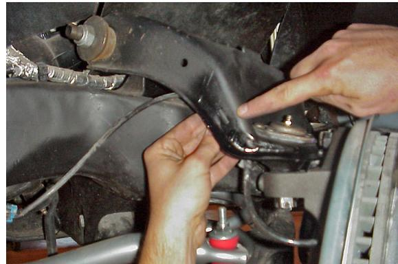
13. Remove the two 18mm bolts attaching the brake caliper mounting bracket to the spindle. DO NOT remove the caliper from the mounting bracket.
