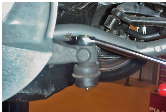
40. Attach the sway Bar end links to the lower control arms. Use a 13mm socket and open-end wrench to tighten the hardware just until grommets begin to bulge.
