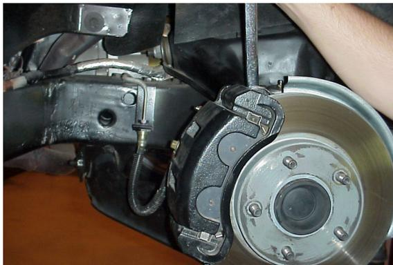
14. Remove the caliper from the spindle assembly by sliding it up and away from the brake motor, ensure not to stretch or damage the rubber brake hose. When the brake caliper is removed, do not allow it to hang unsupported from the brake line. Support the caliper with a piece of wire or cord to prevent damage to the brake line.
