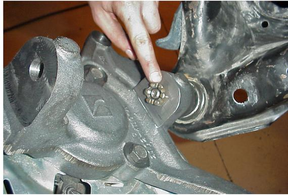
34. Use the floor jack to lift the lower control arm and spindle assembly. Push the upper control arm down until the upper ball joint stud protrudes through tab in the spindle. Thread the castle nut onto the upper ball joint stud and torque the castle nut to 79 ft lbs. Align the slots in the castle nut with the hole in the stud and install a new provided cotter pin. Bend one leg of the cotter pin around the stud to secure nut.
