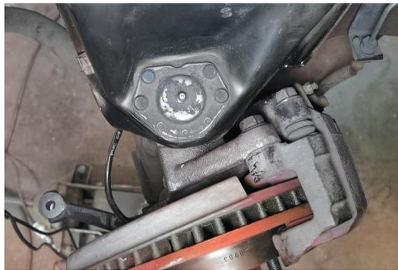
39. Place the tie-rod end stud into the steering arm of the spindle until it protrudes through the top of the tapered hole. Thread the castle nut onto the tie-rod end stud and torque to 39 ft lbs. Align the slots in the castle nut with the hole in the stud and install a new provided cotter pin. Bend one leg of the cotter pin around the stud to secure nut.
