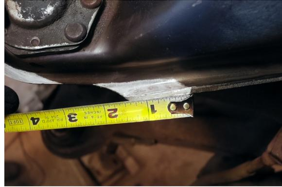
23. Use an angle grinder or die grinder equipped with a cutoff wheel to trim the upper control arm. Grind the surfaces back so that no sharp edges are present.
