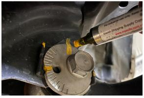
14. Break loose but do not remove the 22mm bolts securing the lower control arm to the frame. Loosen in small increments until the lower control arm can swing downward. Support the lower control arm to prevent it from swinging down too quickly.
