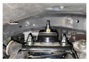
29. Attach the lower coilover mount to the lower control arm using the original nut and bolt. Once the suspension is stabilized, torque 61 ft lbs.
