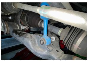
13. Mark the alignment of the camber and caster adjustment bolts securing the lower control arm to the frame. This will help keep the alignment close to the original settings when installing the control arms.
