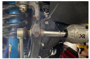
10. Disconnect the tie rod by removing the cotter pin and 19mm castle nut. Strike the designated area on the spindle to dislodge the tie rod.
