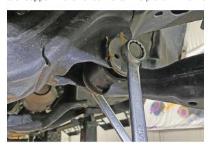
15. Remove the three top mount 14mm nuts and remove the strut from the vehicle. Hold the strut to avoid dropping it. Additional adjustment of the spindles' position may be necessary to pull the strut down. Do not separate the joints of the axle by pulling on the spindle too much.
