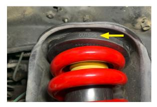
27. Reference the markings made before disassembly and ensure the top mount is oriented in the same position. Torque the supplied Nyloc nut onto the coilover. Torque to 20 ft lbs.
