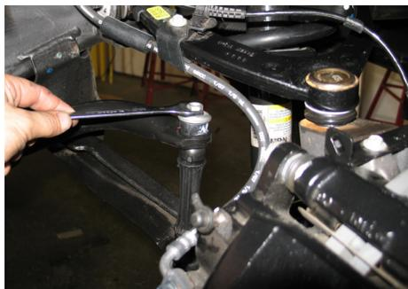
13. Once all the mounts have been un-bolted, hold the spindle assembly while slightly pushing down, dislodging the bottom spring/strut assembly from its perch, paying extra attention to not damage or over extend brake hoses.
