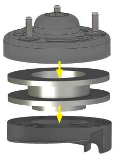
19. Place the Belltech upper strut spacer on the strut. Use the alignment pin as a guide to install the spacer in the correct direction
