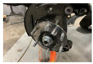
14. With a 15mm wrench, remove the three top mount nuts holding the strut to the chassis. Lower the control arm assembly to gain clearance for the strut to be removed from the vehicle. Next, remove the OEM lower strut bolts to ease the installation later.
