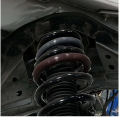
33. Remove the rear strut assembly from the vehicle.
