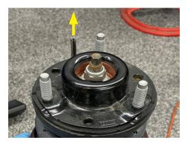
35. Place the top mount studs through the upper strut spacer and fasten the spacer on the strut using original hardware.
