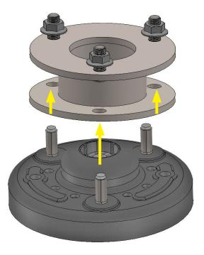
36. The taper on the strut spacer will have the shorter side facing towards the front of the vehicle and the taller side to the rear. Torque the spacer to the strut to 41 ft lbs.
