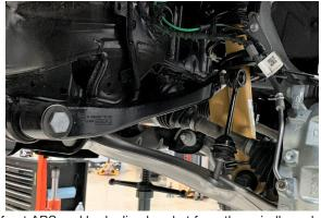
10. Using a 10mm wrench, detach the front ABS and brake line bracket from the spindle and remove the bracket from the chassis. Also remove the 8mm bolt to detach the wheel speed sensor from the spindle. Secure the wire assembly away from the working space.
