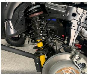
39. Reattach the lower strut bolt and torque to 350 ft lbs.
