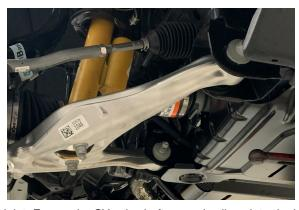
23. Attach the spindle to the upper ball joint. Ensure the CV axle shaft properly aligns into the hub. Torque the upper ball joint nut to 46 ft lbs.
