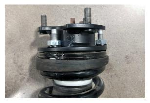
36. Mount the strut and spacer assembly on the vehicle.
