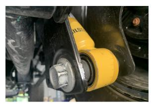
32. Remove the 15mm upper strut mount bolts.
