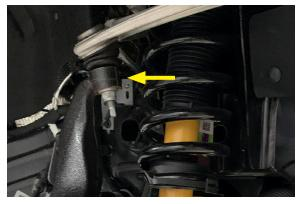
13. With a 36mm socket, remove the CV axle nut. Ensure the axle is dislodged from the spindle by striking the center of the axle with a punch and hammer. Ensure the threads are not damaged in the process.
