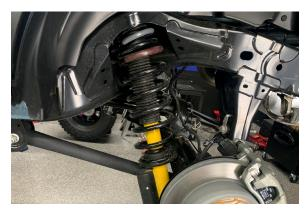
38. Attach the lower strut bolt and nut, torque to 350 ft lbs.
