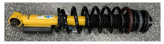
34. Attach the strut spacer onto the top mount by aligning the bolts and guide pin.
