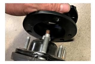
20. Secure the spacer with the split washers and M10x1.5mm nuts. Spin the nuts until snug then tighten using an open ended wrench or thin wall socket.
