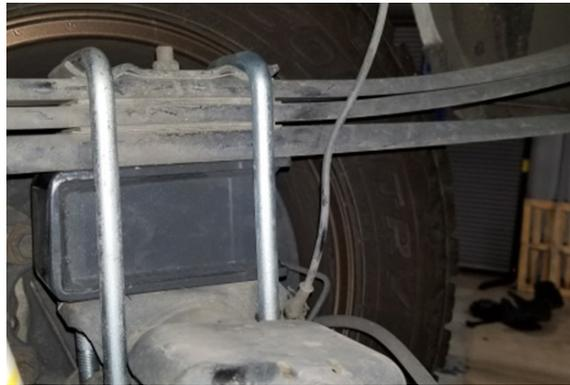
33. Use the jack to apply slight pressure at the rear axle to keep the pin aligned. Install the supplied Belltech U-bolts and tighten in a crossing pattern; then torque to First Pass: 59 ft lbs., Second Pass: Loosen 180 degrees, Third Pass: 59 ft lbs., Final Pass: 120-140 degrees.
