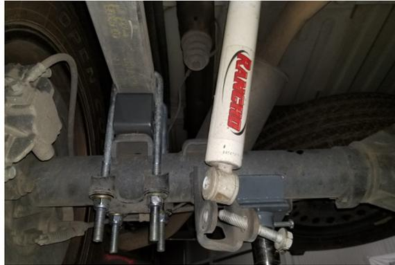
31. Loosen the 21mm U-bolt nuts evenly until removed. Detach the original U-bolts to remove the factory blocks. Slowly lower the axle using the jack to install the new Belltech lift blocks.
