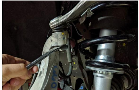
16. The struts must be removed.
