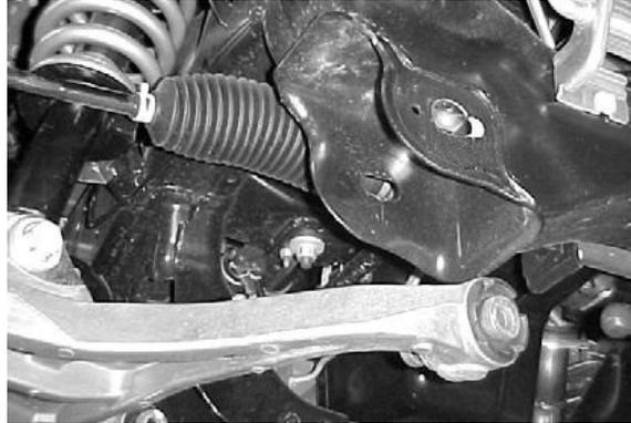
2. Scribe a 1/2" line inward from the edge of the factory alignment slot in the chassis. This must be done to all four slots on each side of the vehicle.
