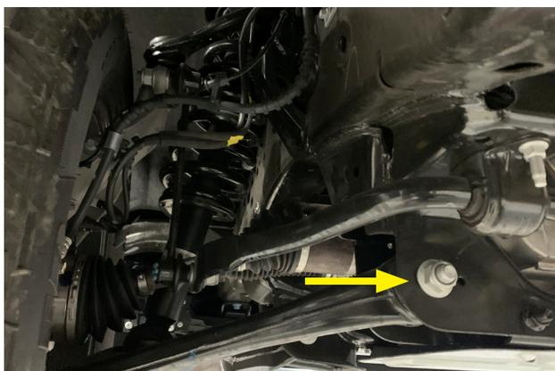
11. Remove the two 18mm nuts securing the lower strut mount to the control arm.
