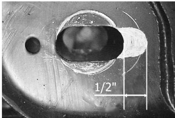
3. Use a die grinder with a carbide cutting tip to carefully elongate the slot towards the center of the vehicle. Do not elongate beyond the 1/2" outlined as this will allow the control arm to contact the frame.
