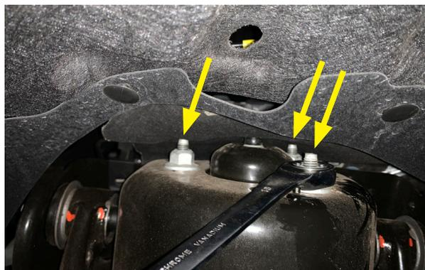
21. Attach the lower strut mount to the lower control arm using the supplied flanged bolts and Nyloc nuts. Torque the supplied nuts to 66 ft lbs.
