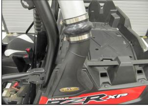
**12.** Install the Hump Hose (#7) and Aluminum Intake Tube (#2) onto the Fender adapter. Loosely install two #48 Clamps (#10) onto the Hump Hose.
