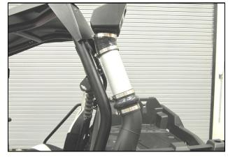
**14.** Install the Snorkel Inlet and elbow onto the Intake tube. Align the assembly into the desired position and tighten all of the Clamps.
