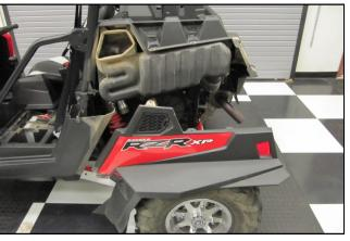
**2.** Starting on the Drivers side first, remove the nine T-27 Torx head screws holding the fender in place. Remove the fender and place it on a work bench.
