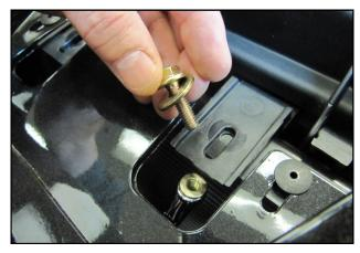
7. Using a 10mm box end wrench and socket, remove the two front airbox nuts and bolts in the core support.
