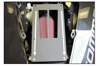
**19.** Install the Pre Filter Tray (#5) onto the Airbox using two 1/4 20 Putter Heads and Flet Western as shown
