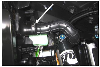
**3.** Loosen the firewall side clamp of the air inlet tube located in the passenger side front wheel well.
