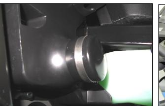
**28.** Install the 2" cap and # 28 Hose Clamp onto the fire wall in the passenger side inner fender (See step **3.**).
