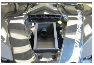
**12.** Position the Airaid Intake assembly into the vehicle and the coupler onto the throttlebody.
