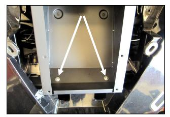
**13.** Secure the Intake assembly to the core support using the two 1/4-20 Button Head Screws (#12), 1/4" Flat Washers(#13), and 1/4-20 Flange Nuts (#14).
