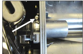
**4.** Remove the center section of the hood to gain access to the airbox assembly.
