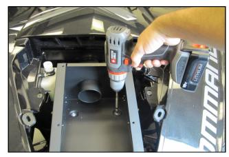
**15.** Using the drill and a 8mm socket, drive the Self Drilling Screws (#15) with a 1/4" Flat Washer into the cross member.
