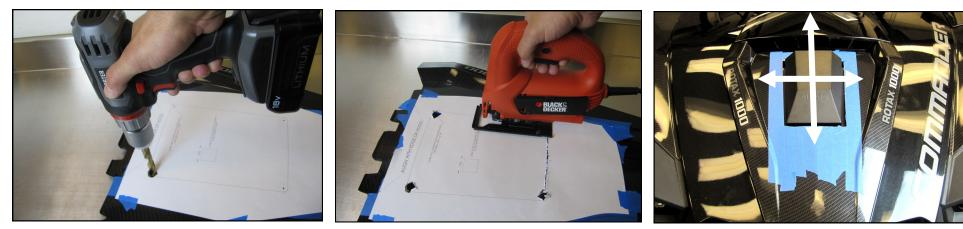
**22.** Using a 1/8'' bit, drill out four pilot holes in the hood followed by a 1/2'' bit to finish.
