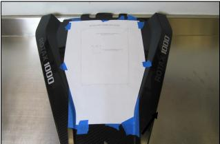
**21.** Prepare the hood for cutting by laying tape strips side by side all across the center section for scratch protection
