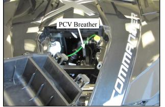
**8.** Disconnect the PCV Breather from the airbox lower half and remove it from the vehicle.
