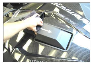
**27.** Compress and install the Foam Pre Filter (#7) into the Hood Scoop.
