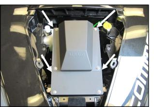
**20.** Mount the Hood Scoop onto the Airbox assembly a shown using four sets of 1/4 20 Button Heads and
