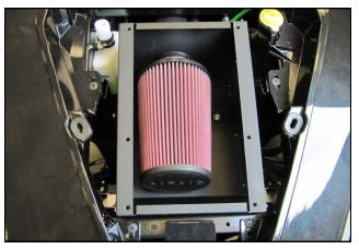
**18.** Slide the Airaid Premium Filter onto the inner Airbox tubing and tighten the Clamp.
