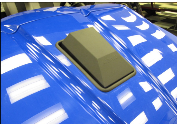
21. Lower the hood down onto the vehicle and secure it. Align the Hood Scoop from left to right inside of the cut out . Raise the hood, secure the Bolts and re connect the battery.
