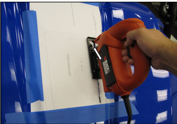
15. Using a jig saw, cut out the center section of the hood.
