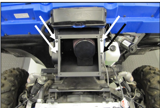
11. Insert the Airbox outlet into the Silicone coupler and tighten the Clamps. Mount the airbox to the vehicle by reusing the factory hardware from step one.
