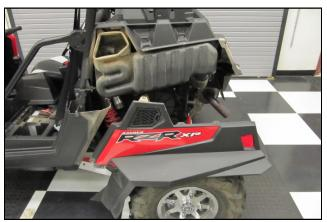
**2.** Starting on the Drivers side first, remove the nine T-27 head screws holding the fender in place. Remove the fender and place it on a work bench.
