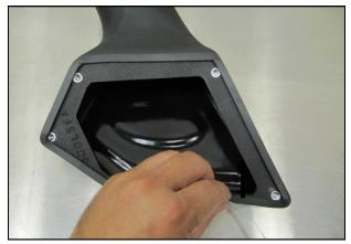
7. Prepare the mating surface of the Fender Adapter (#2) for the Foam Gasket Tape (#10) by cleaning with a prep solvent. Apply the gasket tape along the outside edge of the Fender Adapter as shown, avoiding the bolt holes.
