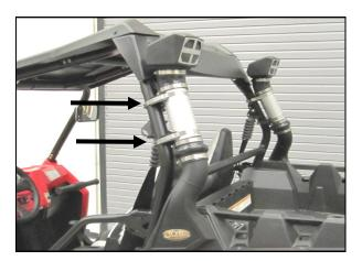
**15.** Secure the snorkel assemblies to the roll cage using the Tube Mounts (#9) and #68 Clamps (#12). Align the Snorkels to each other for symmetry.
