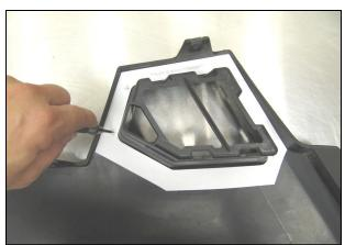
**4.** Cut out the paper Template. Align it with the edges of inner fender, and punch the four pilot holes. Be careful with the Template as it will be re used on the passenger side fender too.
