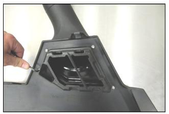
**8.** Attach the Fender Adapter to the outside of the factory Fender using four 1/4-20 button head screws (#14).
