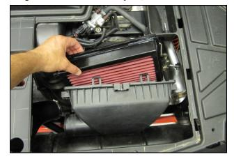
17. Apply the supplied silicone grease (#15) to both sides of the sealing flange on the Airaid Premium Filter. Install the filter as shown, flange first, with the domed portion facing away from the engine.
