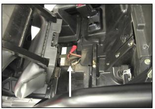
**1.** Place the range selector in Park and remove the drivers seat from the vehicle. Disconnect the negative terminal on the battery.
