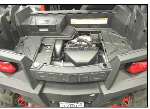
**16.** Remove the access hatch in the bed and remove the factory air filter from the airbox.
