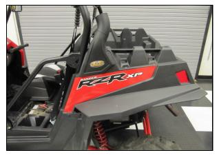
**9.** Re install the fender onto the vehicle, reusing the nine fasteners from step 2.
