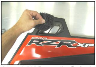
**3.** Remove the OEM filter cover and pre filter from the fender and set aside. They will not be reused.
