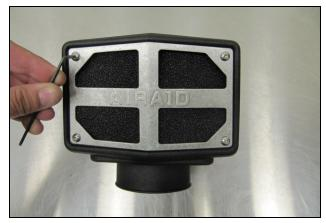
11. Install the Snorkel Screen (#5) onto the Inlet using four 8-32 Button Head Screws (# 13) and a 5/32" Allen wrench
