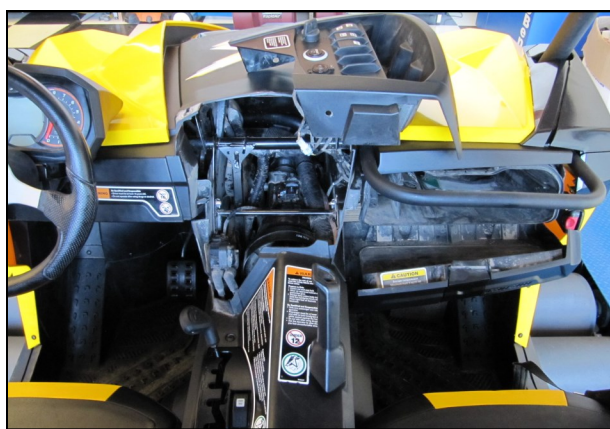
5. Pull the console out and lay it on top of the hood.
