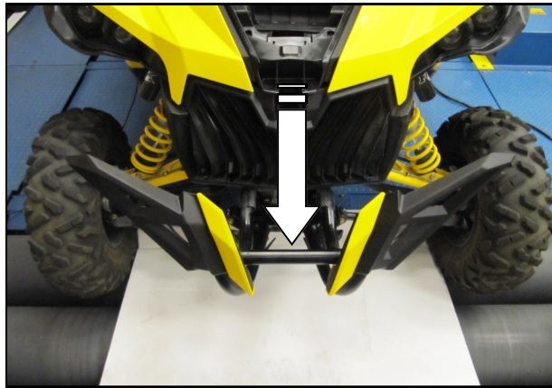
14. Swing the bumper out and away from the front end as far as it will go.
