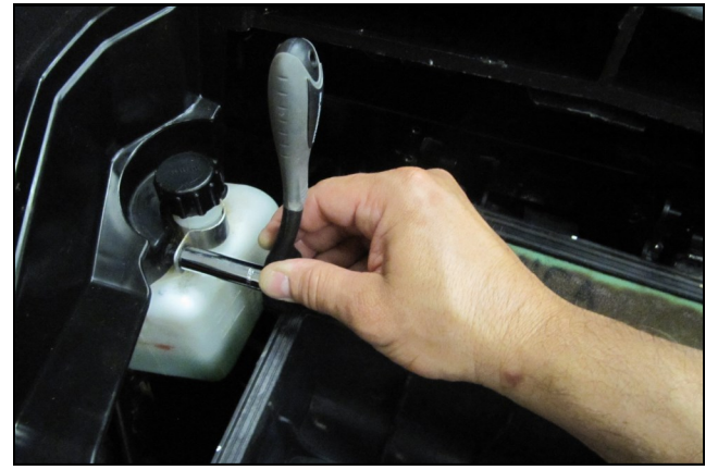
12. Remove one of the 6mm bolts in the coolant bottle bracket to release it and set the bottle inside the compartment.
