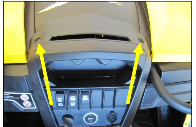
3. Remove the two Torx screws from the top of the center console.
