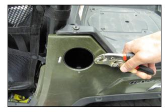
**2.** Using a pair of Locking Pliers, remove the Threaded Studs from the riser tube. Take care not to damage the threads for future installations.
