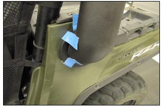
**5.** Determine the optimal position of the Snorkel Tube (#1) for your particular cage configuration. Hold the tube in place and fold the two 8" strips of tape over onto the Snorkel flange.
