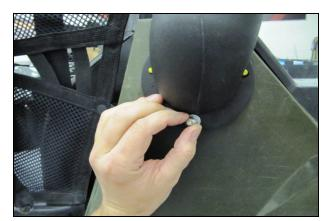
11. Mount the Snorkel tube on to the Threaded Studs and secure using one 1/4-20 x 1" Button Head Bolt (#2), 1/4" Lock Washer (#3), and 1/4" Flat Washer (#4). Do not fully tighten at this time.
