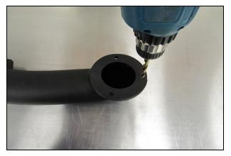
**8.** Remove the Gasket and drill the bolt holes in the Snorkel Flange. Start with 1/8" pilot holes and finish with 5/16" holes.
