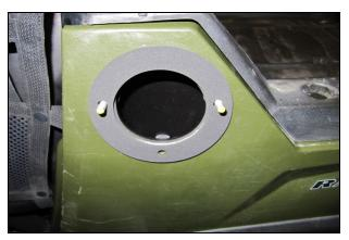
10. Slide the Snorkel Tube Gasket (#6) onto the Threaded Studs.
