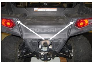
**5.** Using a T-25 Torx driver and a 7/16" wrench, remove the two outer bed bolts.
