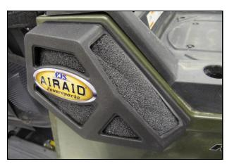
**3.** Insert the Foam Pre Filter (#6) into the Air Scoop as shown. Apply the Airaid Decal as shown.
