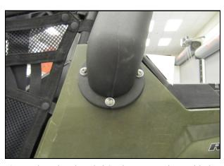
**47.** Replace the Threaded Studs, one at a time, with the remaining 1/4-20 x 1" Button Head Bolts and 1/4" Washers from the previous step. Make all three Bolts final tight.
