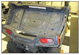
11. Completely remove the bed and set it aside.
