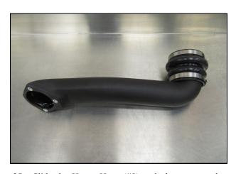
35. Slide the Hump Hose (#8) and clamps onto the Riser Tube (#4) as shown. The #52 Clamp (#19) is to be installed on the Tube side and the #60 Clamp (#20) on the other. Leave the clamps loose for now.
