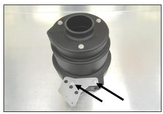
**23.** Mount the Transmission Bracket (#9) to the Air Box using two1/4-20 x 5/8" Hex Bolts, and 1/4" Lock Washers (#15).
