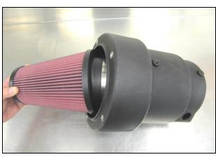
**19.** Insert the Airaid Premium Filter (#1) into the Cold Air Box and onto the Filter Adapter.
