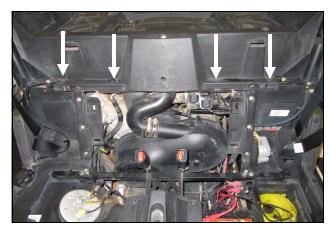
**6.** Using a T-25 Torx driver, remove the four outer bed bolts.
