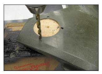
**33.** Drill 5/16" bolt holes in the panel.
