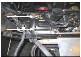
**16.** Remove the two bolts at top of the factory air filter housing and remove the entire housing from the vehi-
