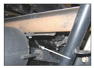
**15.** Loosen the large clamp on the factory intake tube.
