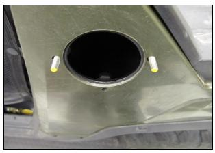
**44** Temporarily install two Threaded Studs (#11), finger tight, into the Riser Tube as shown.
