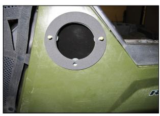
**45.** Slide the second Snorkel Tube Gasket on to the Threaded Studs.
