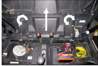
**3.** Remove the front engine cover by rotating the two twist locks counter clockwise and lifting out.
