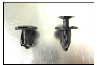
1. Many of the panels needing to be removed for this installation are held in place with the use of nylon rivets. Nylon rivets are reusable if care is taken during their removal and installation. Using a small standard blade screwdriver, gently pry up on the center post until the entire rivet can be pulled freely from the panel. Rivet installation is the opposite.
