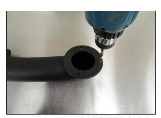
**42.** Remove the Gasket and drill the bolt holes in the Snorkel Flange. Start with 1/8" pilot holes and finish with 5/16" holes.
