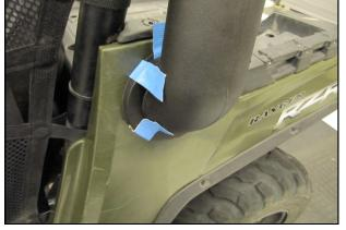
**39.** Determine the optimal position of the Snorkel Tube (#30) for your particular cage configuration. Hold the tube in place and fold the two 8" strips of tape over onto the Snorkel flange.
