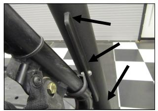
**48**. The Snorkel Tube has a large mounting tab to accommodate many cage options. Determine the best location for attachment and drill a 5/16" hole. Use the supplied Loop Clamp and the remaining 1/4-20 hardware (#31,14 & #17) to secure the Snorkel Tube.
