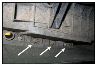
**8.** Under side view of three bed screws to remove.
