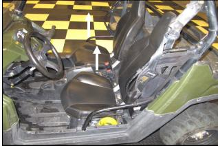
**2** Place the range selector in Park. And remove both driver and passenger seats. Disconnect the negative terminal on the battery.
