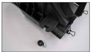
7. Remove the factory grommet and sleeve from the factory lower air filter housing.
