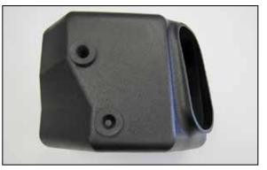
6. Remove the two mounting grommets from the factory lower air filter housing and install them into the AIRAID<sup>®</sup> housing as shown.
