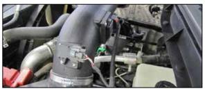
19. Reconnect the mass air and temperature sensor electrical connections.
