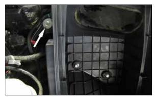
4. Remove the bolt that secures the lower air filter housing to the inner fender and then pull firmly up to release the lower housing from the mounting grommets and remove it from the vehicle. **NOTE: This bolt will be reused in a later step.**  5. Remove the gasket from the factory fresh air intake.
