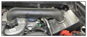
18. Install the AIRAID® intake tube assembly into the coupler at the turbo and filter adapter, adjust the tube for best fit and then secure with the provided hose clamps.
