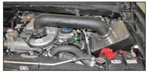
20. Double check your work! Make sure there is no foreign material in the intake path. Make sure all clamps, hoses, bolts, and screws are tight. Double check the hood clearance! **Reconnect the negative battery cable!**
