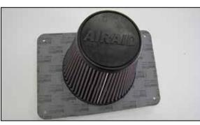
11. Place the housing lid gasket onto the lid and then install the AIRAID® air filter and secure with the provided hose clamp.
