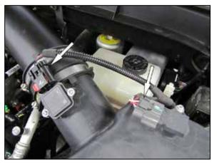
2. Disconnect the mass air sensor and inlet air temperature sensor electrical connections.
