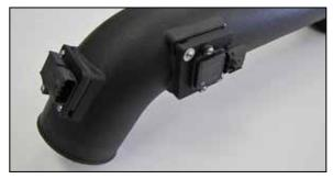
17. Install the sensor assemblies into the AIRAID® intake tube and secure with the provided hardware. NOTE: Be sure the mass air sensor is installed in the correct direction.
