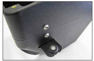
8. Install the grommet and sleeve from the previous step into the provided mounting bracket, then install the mounting bracket through the AIRAID® air filter housing and secure with the provided hardware.
