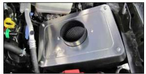
12. Install the lid assembly onto the AIRAID® air filter housing and secure with the provided hardware.
