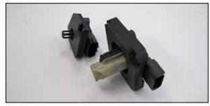
16. Install the factory sensors into the provided sensor adapters and then install the provided gaskets onto the adapters.
