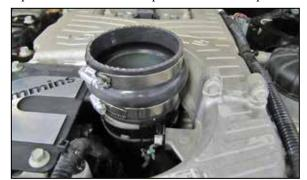
14. Install the provided hump coupler onto the turbo inlet and secure with the provided hose clamp.
