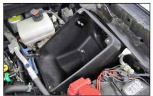
9. Install the AIRAID<sup>®</sup> air filter housing onto the mounting studs on the inner fender and secure with the factory bolt removed in step #4.
