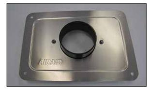
10. Install the filter adapter onto the air filter housing lid and secure with the provided hardware.
