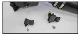
15. Remove the mass air sensor and temperature sensor from the factory air filter housing.
