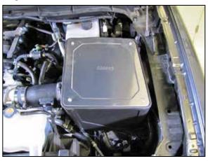
19. Install the air filter housing gasket and lid and secure with the provided hardware.
