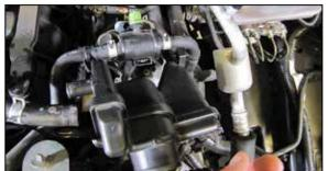
6. Disconnect the crank case vent lines and then loosen the clamp that secures the canister to the intake tube and remove the canister.
