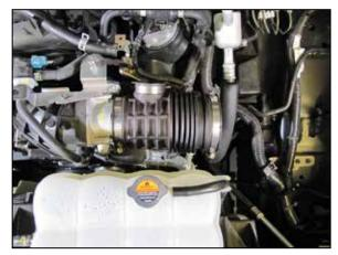
7. Loosen the hose clamp and then remove the factory intake tube from the vehicle.
