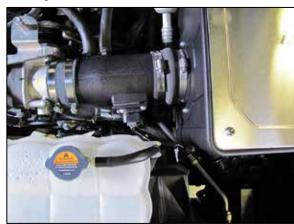
20. Reconnect the mass air sensor electrical connection.
