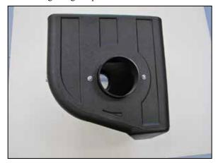
9. Install the filter adapter into the AIRAID® air filter housing using the provided hardware.
