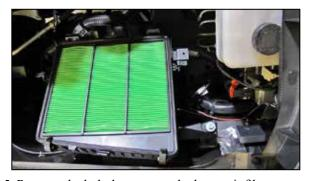
5. Remove the bolt that secures the lower air filter housing and then remove the housing from the vehicle. **NOTE: AIRAID recommends that customers do not discard factory air intake.**
