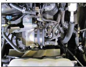
14. Install the provided coupler onto the throttle body and secure with the provided hose clamp.
