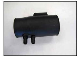
13. Install the two vent fittings into the AIRAID $^{\text{@}}$  intake tube as shown.
