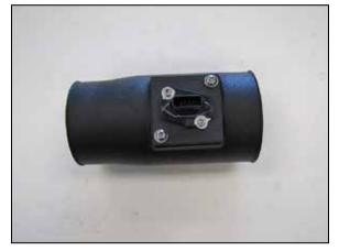
12. Install the mass air sensor assembly into the AIRAID® intake tube and secure with the provided hardware.
