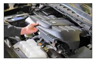
3. Lift up the engine cover and remove it from the vehicle.
