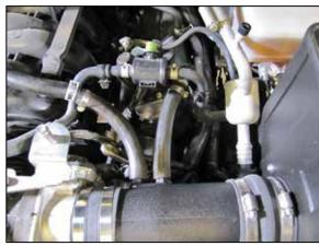
18. Install the hose menders into each vent hose and then connect the hoses to the factory vent hoses and to the fittings installed into the AIRAID® intake tube.
