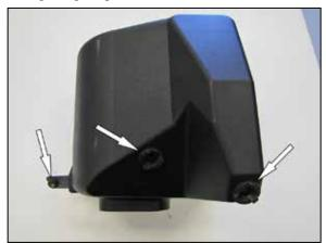
10. Remove the three mounting grommets from the factory air filter housing and install them into the AIRAID® housing as shown.
