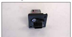
11. Remove the mass air sensor from the factory air filter housing and install it into the AIRAID® mass adapter and secure with the provided hardware. Apply the provided gasket onto the bottom of the adapter.
