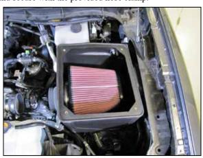
15. Install the AIRAID® air filter housing into the vehicle and then install the air filter onto the filter adapter and secure with the provided hose clamp.
