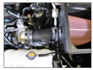
16. Install the provided hump coupler onto the AIRAID® intake tube and then install the intake tube into the vehicle, adjust the tube for best fit and then secure with the provided hose clamps.
