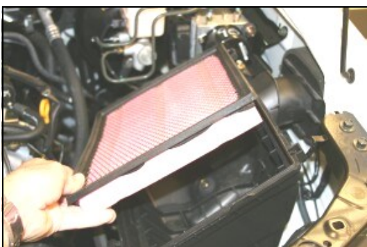
7. Remove the factory air filter.
