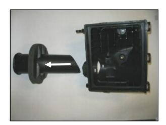
**4.** Remove the factory air box base from the vehicle. Using a flat blade screwdriver, unsnap and remove the factory tube from inside the air box base. Reinstall the factory air box base and the bolts into the
