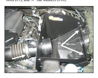
**8.** Install the Quick Fit Panel assembly onto the factory air box base using the factory clips. Slip the factory intake tube over the air filter adapter, and then tighten the factory hose clamp.
