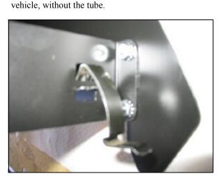
**7.** Remove the clip from the factory air box lid and install it in the Quick Fit Panels as shown.
