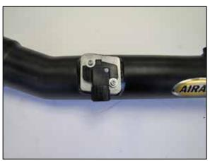
11. Remove the mass air sensor from the factory housing and then install it into the AIRAID® intake tube and secure with the provided hardware.
