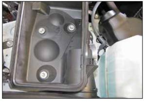
6. Remove the factory air filter from the lower housing and then remove the 3 bolts that secure the housing to the inner fender and remove the housing from the vehicle
