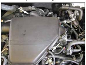
4. Disconnect the fuel pressure regulator vacuum line from the regulator and the crank case vent line from the valve cover.
