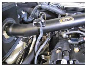
18. Reconnect the mass air sensor electrical connection.
