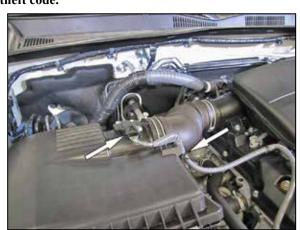
2. Disconnect the mass air sensor and unclip the mass air sensor wiring harness from the factory air filter housing.
