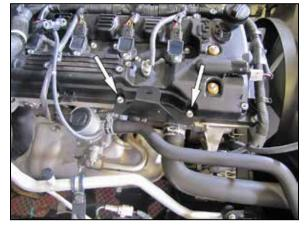
12. Remove two of the bolts shown that secure the cam cover, install the bolts through the provided tube bracket (010114) and then install onto the cam cover and secure.
