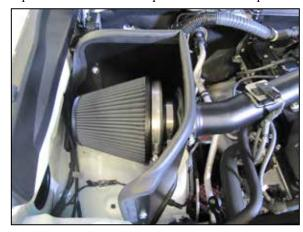
20. Install the filter assembly onto the intake tube and secure with the provided hose clamp.
