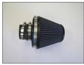
19. Install the filter adapter into the AIRAID® air filter and secure with the provided hose clamp. Install the provided coupler (AIR-KITRDCR05) onto the filter adapter and secure with the provided hose clamp.
