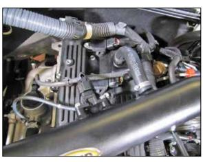
17. Install the provided crank case vent line onto the valve cover port and onto the AIRAID® intake tube. Install the vacuum switch onto the AIRAID® intake tube and secure with the provided hardware.
