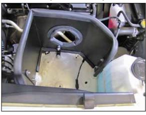
14. Install the heat shield onto the inner fender and secure with the hardware provided and the factory nut removed in step #7.
