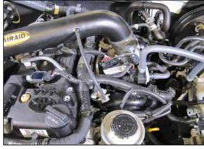
16. Install the provided fuel pressure regulator vent line onto the regulator and onto the AIRAID® intake tube.
