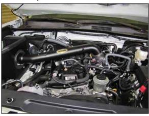
15. Install the AIRAID® intake tube into the coupler at the throttle body and align with the mounting bracket. Secure the tube with the provided hose clamp and hardware.
