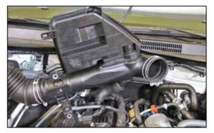
5. Release the upper air filter housing clips, loosen the hose clamp securing the intake hose to the throttle body, lift the intake system and unclip the wires secured to the intake system then remove the system from the vehicle.
