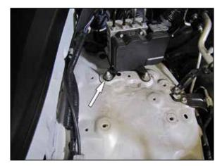
7. Remove the nut shown from the ABS mounting bracket.
