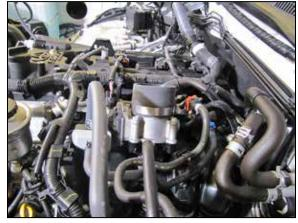
13. Install the provided coupler onto the throttle body and secure with the provided hose clamp.
