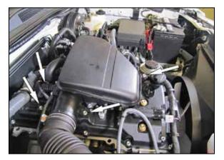
3. Remove the bolts that secure the vacuum switch to the back of the intake plenum, remove the three bolts that secure the intake plenum to the engine.
