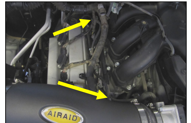
40. replace the OEM vacuum line on the fuel pressure regulator with the supplied 20 1/2" 1/8" line (#12). Connect the 1/8" line to the small Fitting on the Intake tube.
