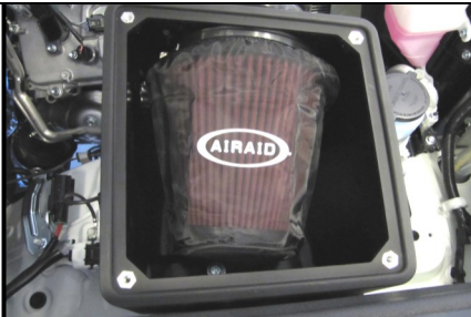
42. Place the Gasket (#10) onto the underside of the Air Box Lid (#4) and peel off the protective film. Mount the lid on the Air Box using four 1/4-20 x 1/2" Button Head Bolts (#18), and 1/4" Flat washers (#19).
