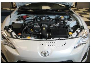
With help from an assistant. The inlet can be removed without removing the entire bumper cover. Simply remove all of the topside fasteners and pull back on the cover. Have an assistant remove the two 6mm bolts in the tube and remove.
