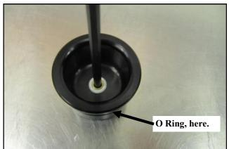
Apply a thread sealer to the threads of the Brass plug and insert it into the Resonator Tube Plug. Slide the O Ring onto the plug and into the groove. Install the Plug Assembly into the Intake tube port and secure using the #24 Clamp. It should be noted that the Aluminum Plug is designed to accept many 1/16 NPT N2O foggers.
