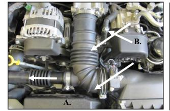
1. Disconnect The Negative Battery Terminal! Loosen the clamps on the throttle body and the airbox outlet. A. Loosen the resonator tube clamp and disconnect it from the intake. B. Compress the spring clamp on the crank case breather line and disconnect it. Remove the intake tube from the vehicle.
