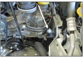
**5.** Install the CAB Mount into the airbox bracket on the inner fender. Hand tight is sufficient.
