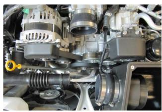
10. Place the Hump Hose and two #52 Clamps onto the Filter Adapter and the Reducer with one #52 and one #44 Clamp on the throttle body. Leave the clamps loose
