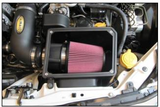
13. Install the Airaid Premium Filter onto the Filter 14. Carefully install the Gasket onto the Air Box Lid. Adapter.
