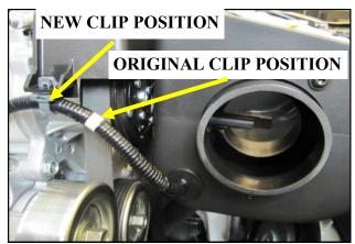
9. Route the MAF harness into the Airbox and reconnect the sensor inside. Seal off the access port with the Grommet from step 9. Relocate the plastic clip on the wire harness 1 1/4" back to take up any slack that might allow contact with the accessory belt.
