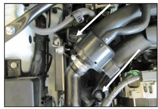
Install Option One: Resonator Delete. Loosen the resonator tube clamp and disconnect it from the Intake. Remove the two 6mm bolts in the diaphragm housing and pull the sound tube out of the fire wall. Remove the entire resonator as an assembly.
