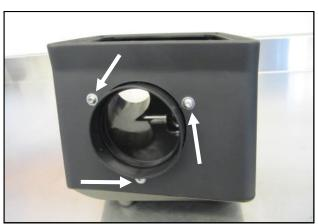
7. Mount the Filter Adapter to the Cold Air Box, as shown, using three 1/4-20 x 1/2" Button head Bolts and 1/4" Flat Washers.
