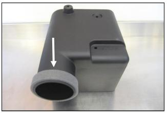
**6.** Apply the self adhesive, Foam Weatherstrip onto the air inlet on the Cold Air Box .
