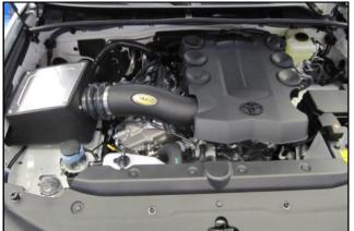
Make sure there is no foreign material in the intake path. Make sure all clamps, hoses, bolts, and screws are tight. Double check the hood clearance!
