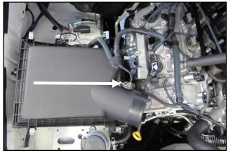
**3.** Disconnect the Mas Air Flow sensor and remove the factory airbox top and air filter.
