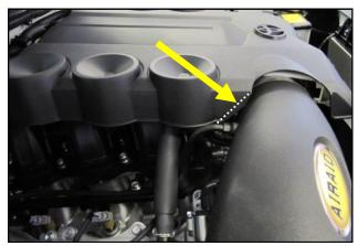
13. Place the engine cover back on top of the motor and note the location where it comes in contact with the Airaid Intake Tube. Remove the cover and trim the edge approximately 1/8" and reinstall.
