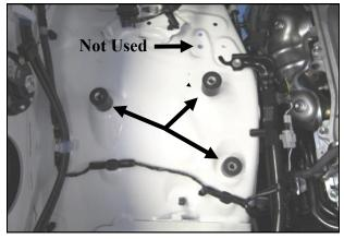
**5.** Install the three M8 CAB Mounts , hand tight, into the weld nuts on the inner fender as shown. Note: One of the original air box mounting holes is not re used. Note: It may be necessary to chase the threads first using the factory bolts in order to clear out the factory undercoat.
