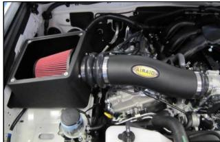
14. Install the Airaid Premium Filter onto the Filter
