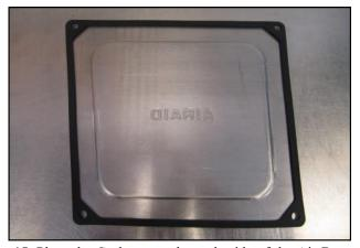
**15.** Place the Gasket onto the underside of the Air Box Lid and peel off the protective film. Mount the lid on the Air Box using four 1/4-20 x 1/2" Button Head Bolts, and 1/4" Flat washers.
