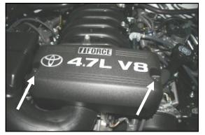
1. **Disconnect the negative battery cable.** Using a 10mm socket, remove two nuts and the engine beauty cover. Set them to the side for now, they will be reinstalled in step #14.
