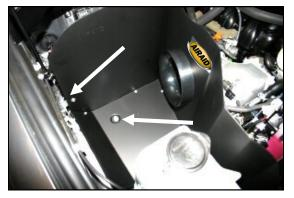
**8.** Install the **CAD** assembly into the vehicle. Align the hole in the bottom over the captured nut in the fender well. Install one 6mm hex bolt (#16), and washer (#14). Leave loose for now. Next reinstall the factory bolt removed in step #6, thru the bracket, into the ground anchor in the fender well. This bolt can be tightened now.
