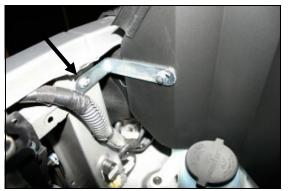
**13.** Fasten the #203 bracket (#26) to the existing hole in the radiator support using one  $1/4-20 \times 1/2$ " button head bolt (#13) washer (#14), and serrated nut (#15). Tighten all nuts and bolts that hold the **CAD** to the vehicle at this time.
