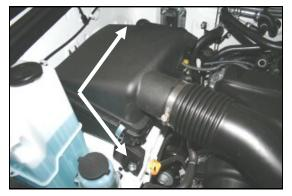
**5.** Using a 10mm socket, loosen the two bolts that anchor the factory airbox to the inner fender-well. One is on the front of the airbox, and the other is on the rear. Pull the factory intake tube away from the throttle body and remove the com-
