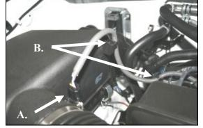
**3. A**.) Squeeze the tab on the Mass Air Flow (MAF) sensor wiring connector and disconnect it from the sensor. **B**.) Squeeze the tabs on the bottom of the two wiring harness anchors, and remove them from their respective anchor points.
