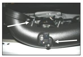
10. Install the 1/8" barbed fitting (#20) into the Airaid intake tube (#2) as shown. Next install the MAF sensor removed in step #9, into the Airaid intake tube and secure it with two 8/32" x 3/8" (#12) button head screws. <u>Do Not Use The Factory Screws!</u>
