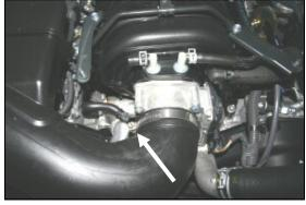
**2.** Using a 10mm socket, loosen the hose clamp that secures the factory intake tube to the throttle body.
