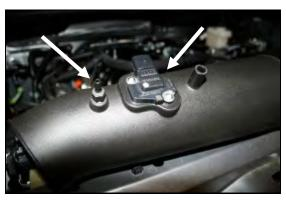
9. Re-install the MAF sensor into the Airaid intake tube (#2) as shown using the supplied 8-32x3/8" button head screws (#12). Do Not Use The Factory Screws! Next install the 1/8NPTx3/16" barbed fitting (#20) into the Airaid tube.
