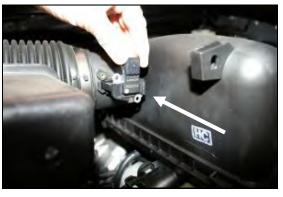
8. Remove two screws, and remove the Mass Air Flow sensor from the factory intake tube. Note the orientation of the sensor in the tube. It will need to be replaced in the same direction in the Airaid tube.
