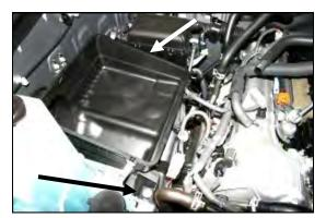
4. Using a 10mm socket, loosen the two bolts that hold the airbox base to the fender well, and
