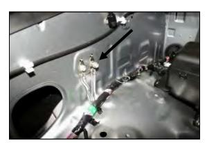
5. Remove the rear ground anchor bolt from the side of the fender well and save it for reuse ir
