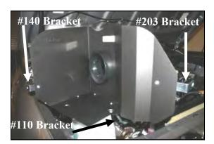
6. Assemble the Cool Air Dam panels (#3 & #4) shown using four 6-32 screws (#9), washers
