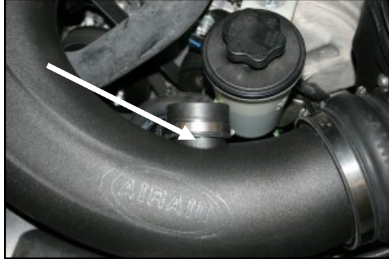
2. Using one of the clamps from the resonator coupler, install the urethane cap onto the intake tube and tighten the clamp.
