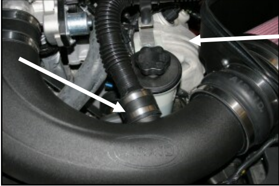
1. Loosen the clamps on the resonator tube coupler and disconnect it from the intake tube. Pull up on the resonator tube to release it from the resonator
