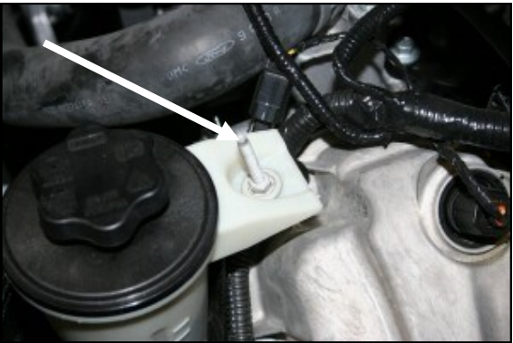
4. Replace the resonator bracket and 6mm bolt with the factory stud removed in step #9.
