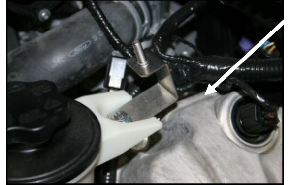
3. Using a 10mm socket, remove the resonator bracket from the power steering reservoir.
