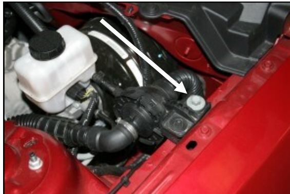
5. Remove the bolt that secures the resonator tube and diaphragm to the left inner fender.
