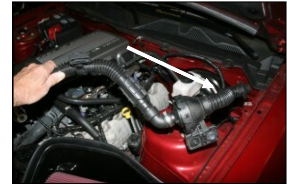
6. Grab the resonator tube between the diaphragm and the firewall and pull up and out to disconnect it from the firewall. Remove the complete resonator assembly from the vehicle.
