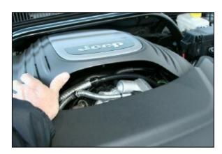
**3.** Carefully lift the engine cover for access to the throttle body. (There are only grommets that hold down the cover, no bolts.)
