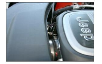
4. A.) Using the 10mm socket, remove the bolt that holds the stock intake system.
