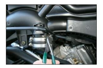
5. Carefully pull the intake towards you and rotate it so the bottom faces you, and cut
