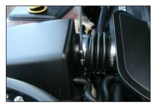
1. Disconnect the negative battery cable. Loosen hose clamp on air cleaner box lid. Carefully twist and remove the breather hose from the lid.
