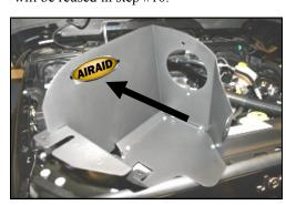
11. Assemble the Cool Air Dam panels (#3 & 4) as shown, using the seven 6-32 screws (#10), flat washers (#11), and keps nuts (#12). Apply the Airaid Decal as shown.
