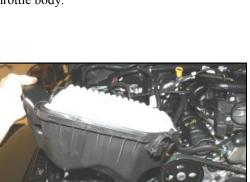
**5.** While rocking the factory air cleaner base back and forth, pull up, and remove it from the vehicle. There are no bolts holding it down, just grommets.
