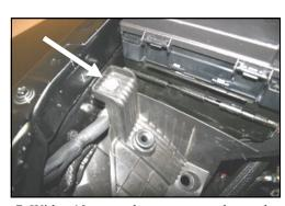
**7.** With a 10mm socket, remove and save the bolt from the factory plastic air cleaner mount. It will be re-installed in step #12.
