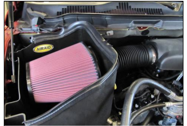
12. Install the Airaid Premium Filter onto the Filter Adapter inside the Cool Air Box. Install the Weatherstrip onto the Cool Air Box as shown, with the contour rolling away from the Filter. Apply the Airaid Bubble Decal inside the Airbox as shown.
