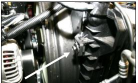
**4.** Gently rock the airbox base back and forth while pulling up, to remove it from it's mounting grommets, and remove it from the vehicle.
