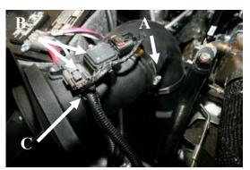
**13. A)** Slide the rubber elbow over the Airaid filter adapter, install one #80 hose clamp (#20), and tighten the hose clamp. **B)** Using three 8-32x1/2" button head screws (#13), reinstall the factory Mass Air Flow sensor, and temperature sensor into the Airaid filter adapter. **Do Not Use The Factory Screws! C)** Reinstall the wiring harness anchor into the hole in the filter adapter just below the temperature sensor.
