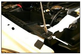
**3.** Using a 10mm socket, remove the nut that holds the front of the airbox base and grommet assembly to the radiator support.
