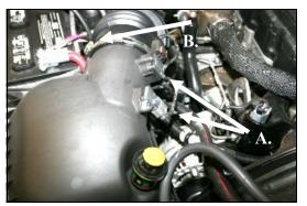
1. Disconnect the negative battery cables. A) Using the supplied #20 Torx bit, remove two screws from the Mass Air Flow sensor, and one screw from the temperature sensor. Remove both sensors and the wiring harness anchor from the airbox lid, and set them aside. C) Loosen the hose clamp that holds the factory intake tube to the airbox lid.
