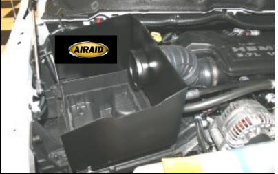
4. Install the Quick Fit Panel (#2) by slipping it into the factory intake tube, and then sliding it over the tabs on the factory airbox base. Adjust it for fit on top of the airbox base, and re-latch the 4 clips to hold the Quick Fit Panel securely in place. Apply the Airaid Foil Decal onto the Panel as shown.
