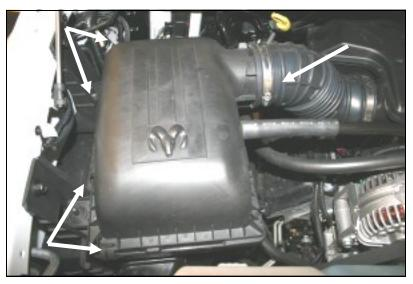
**2.** Unlatch 4 clips that hold down the factory airbox lid. Loosen the hose clamp on the factory intake tube where it connects to the airbox lid, then remove the lid.
