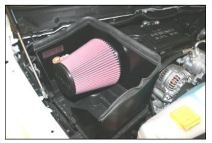
6. Install the Airaid Premium Filter (#1) onto the tube of the **Quick Fit Panel** as shown, and tighten the hose clamp. Now install the weather strip (#3) on top of the **Quick Fit Panel**. (*Hint: Start with the end of the weather strip at one corner, and work your way around to the other corner*.)
