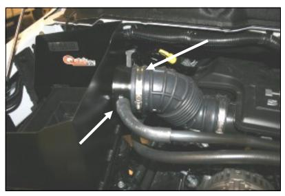
**5.** Slide the factory intake tube all the way onto the **Quick Fit Panel** tube and tighten the hose clamp. Slip the #24 speed clamp(#4) over the factory breather hose and reconnect the factory breather hose to the nipple on the **Quick Fit Panel**. Squeeze the speed clamp to secure the breather hose.
