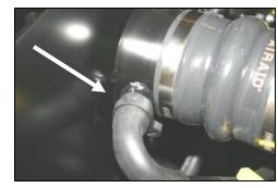
**15.** Slip the #24 speed clamp (#11) over the factory breather hose and re-connect the factory breather hose to the nipple on the Quick Fit Panel . Squeeze the clamp to retain the hose in place.
