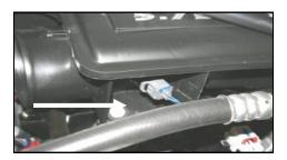
**3.** Squeeze the tab on the connector, and disconnect the intake temperature sensor.
