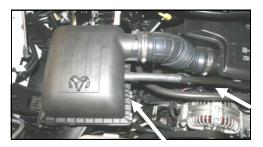
1. **Disconnect the negative battery cable!** Loosen the hose clamp on the resonator. Dis-
