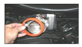
**5.** Remove the factory seal from the throttle body.
