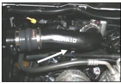
13. (Note: Because factory production tolerances vary, it may be necessary to remove the tape on the wiring loom and pull out 1 1/2" of wire to the temp sensor, and then re-install the tape. Re-connect the wiring harness to the temperature sensor.
