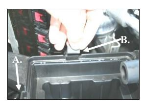
**5.** 2007 Models only: A.) Using a flat blade screwdriver, gently pry and remove one factory clip from the passenger side rear of the airbox base. (see arrow above)
