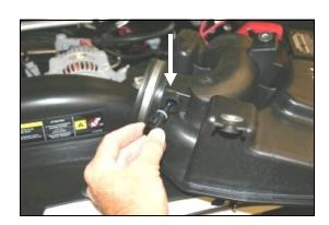
**9.** Carefully twist and remove the **AIT** sensor from the factory resonator.
