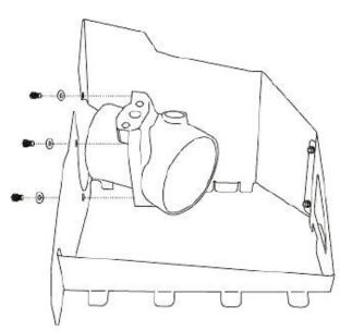
**4.** Assemble the air filter adapter to the cool air dam using the (3) ½-20 bolts and washers provided.
