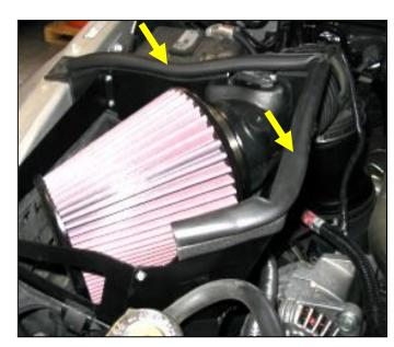
**8.** Mount Airaid Premium Filter to the filter adapter and tighten hose clamp, in addition; press the weather strip onto the top of the Airaid cool air dam. (<u>Hint</u>: start the install at the top corner of the cold air dam & work toward the edges)
