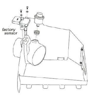
**5.** Fasten the factory sensor on top of the adapter using the (2) 8/32 screws and washers using a 3/32 Allen Wrench.
