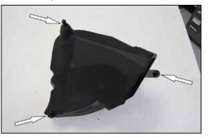
4. Install the provided mounting bracket through the cutout line in the AIRAID<sup>®</sup> air box and then secure with the provided hardware. Install the provided mounting studs onto the bracket and onto the air filter housing as shown.
