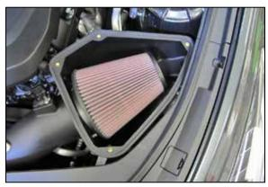
11. Install the AIRAID<sup>®</sup> air filter onto the intake tube and secure with the provided hose clamp.
