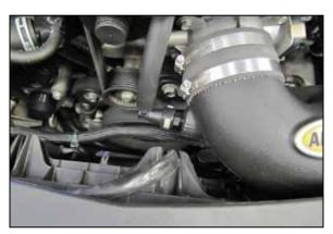
10. Connect the vent line to the quick disconnect fitting installed into the AIRAID® intake tube.
