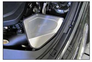
13. Install the provided gasket onto the air box lid,
