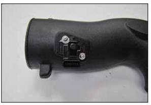
6. Remove the mass air sensor from the factory air filter housing and install it into the AIRAID<sup>®</sup> intake tube using the provided hardware.
