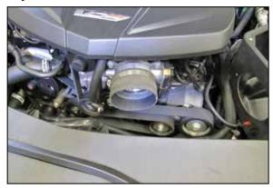
8. Install the provided coupler hose (08761) onto the throttle body and secure with the provided hose clamp.
