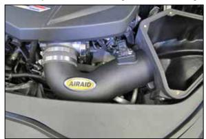
9. Install the intake tube into the air filter housing and then into the coupler on the throttle body, secure the tube to the filter housing using the provided hardware and then secure the tube to the coupler with the provided hose clamp.
