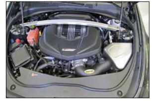
14. Double check your work! Make sure there is no foreign material in the intake path. Make sure all clamps, hoses, bolts, and screws are tight. Double check the hood clearance! **Reconnect the negative battery cable!**
