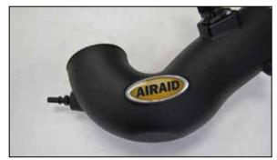
7. Install the provided quick disconnect fitting into the AIRAID<sup>®</sup> intake tube and then apply the provided decal onto the intake tube.
