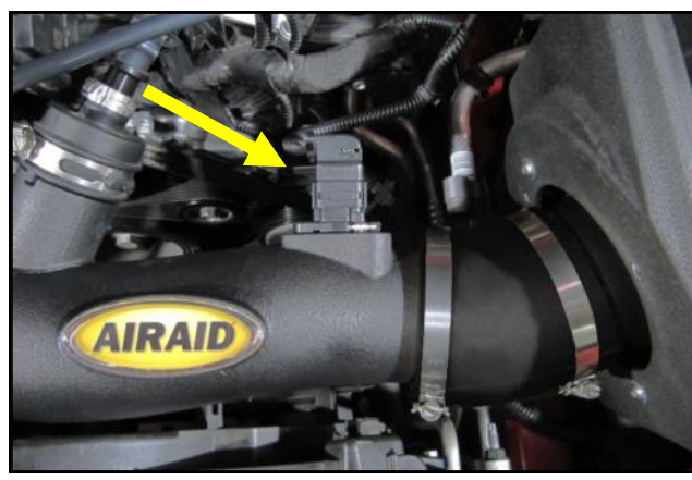
23. Reconnect the Mass Airflow sensor.
