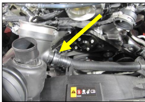
5. Disconnect the resonator tube from the bottom of the factory intake tube.
