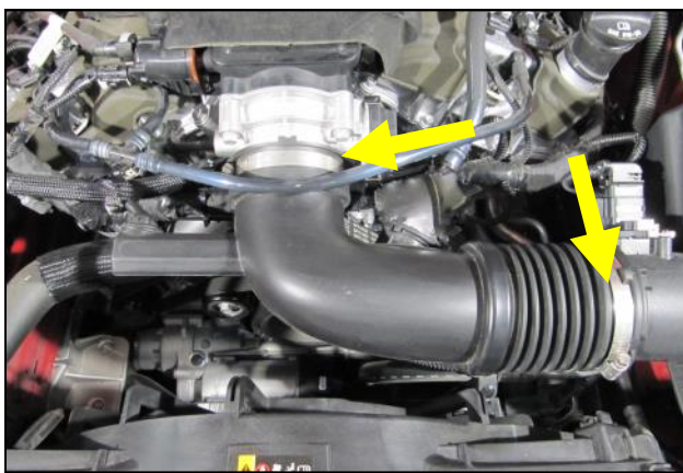
4. Loosen the clamps on the intake tube and remove it from the vehicle.
