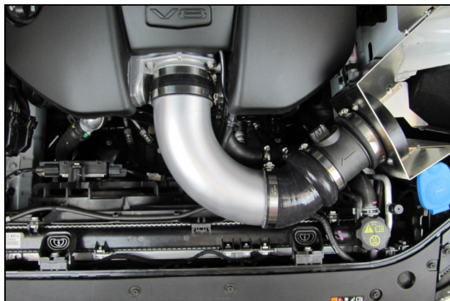
17. Slide the Intake tube into the Hump Hose first, then into the Coupler. Check the positioning of all the components. Adjust if necessary and tighten the Clamps.
