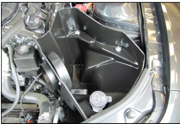
10. Install the Cool Air Box assembly into the vehicle. Slide the airbox grommets and sleeves over the factory studs and secure it using the nuts removed in step 3. Hint: Lifting the washer bottle cap makes for an easier installation.
