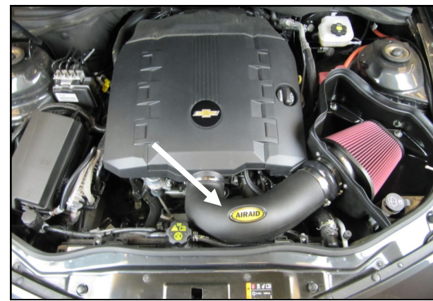
18. Double check your work! Make sure there is no foreign material in the intake path. Make sure all clamps, hoses, bolts, and screws are tight. Double check the hood clearance! Reconnect the negative battery cable. Apply the Airaid Decal onto the Intake Tube.
