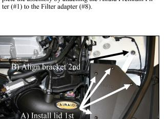
13. A) Attach the Edge Trim (#27) on the Cover (#6) as shown and install the cover using the four Black 1/4-20 Phillips Head Screws. B) Line up the Bracket with the fender bolt hole and secure using the factory hardware. Note: Steps must be performed in order to avoid difficulty with aligning bolt holes.
