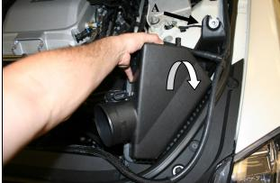
**3. A)** Remove the factory fender bolt securing the airbox assembly. Next pull out the coolant line from atop the airbox lid and gently rotate the airbox assembly towards the front of the vehicle. The airbox assembly is now free and should be removed from vehicle.
