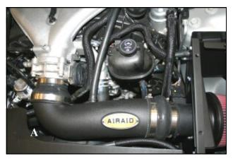
**13.A)** Install the Airaid Intake Tube assembly onto the Mass Air Flow Sensor first, and then onto the throttle body. Adjust for fit, and tighten the hose clamps. **B)** Replace the factory breather line on the valve cover with the 26" Airaid Breather Hose(#11). Secure the breather hose to the intake tube nipple using the black Speed Clamp (#29). Apply the Airaid Bubble Decal onto the Intake Tube as shown.
