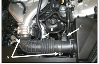
**2. A)** Loosen the hose clamps on the factory intake tube. **B**) Disconnect the breather line and remove the factory intake tube . C) Disconnect the Mass Air Flow sensor.
