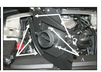
9. A) Transfer the Mass Air Flow Sensor from the factory airbox to the Adapter Panel and secure using two 1/4-20 button Head Screws (#15) and Serrated Nuts (#17). Note: The factory airbox seal on the Mass Air Flow Meter is not to be used in this kit. B) Attach the Weather Strip (# 11) to the curved edge of the MAF Panel. C) Insert the 5/8" hose anchors (#28) into the two horizontal tab holes on the MAF panel.
