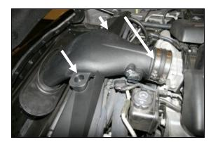
**12.** Install the Airaid Intake Tube assembly onto the throttle body first, and then align the grommets over the factory grommet posts on top of the radiator shroud. Push down on the grommets to seat them on the posts. (*Hint: Use a 1/2" deep socket to help seat the grommets onto the posts.*) Now tighten the hose clamp on the throttle body.
