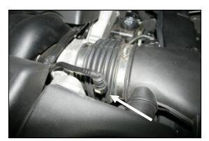
**2.** Squeeze the tabs on the sides of the crankcase breather connector, and disconnect the breather hose from the factory intake tube breather fitting.
