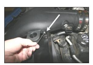
**14.** Tighten all four button head bolts that secure the air dams to the intake tube, and the radiator
