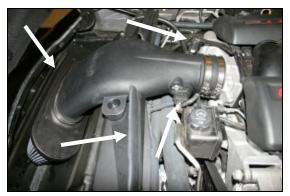
15. Slide the Airaid Premium Filter up onto the end of the intake tube and tighten the clamp. Reconnect the MAF sensor wiring harness and replace the grey security clip. Reconnect the factory breather hose to the breather fitting. Install the weather strip (#6) onto the top of the air dams as shown.
