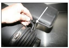
**5.** Remove the factory breather fitting from the factory intake tube and save it for reinstallation in step #6.
