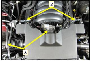
**1.Disconnect The Negative Battery Terminal!** A.) loosen the clamps securing the intake system to the throttle body and the air box.
