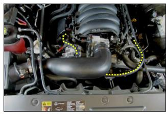
9. Install the Intake Tube and tighten the Clamps. Connect the new breathers to the Barbed Fittings in the Intake tube and the Quick Connect Fittings to the Valve covers .
