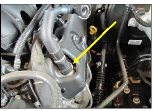
**8.** Remove the valve cover breathers from both sides of the motor and set them aside. They will not be reused.
