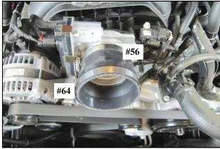
**6.** Slide the Reducer and the #56 and 64 clamps onto the throttle body.
