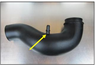
3. Install the Barbed Fitting into the Intake Tube as
